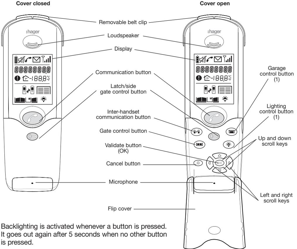
Backlighting is activated whenever a button is pressed. It goes out again after 5 seconds when no other button is pressed.
