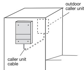
Do not place the products near metal surfaces (screens, fences, gates, etc.) or sources of electromagnetic disturbance:
