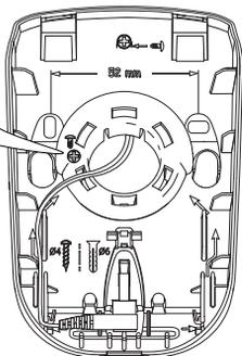
7. Insert the screw here and tighten it.
