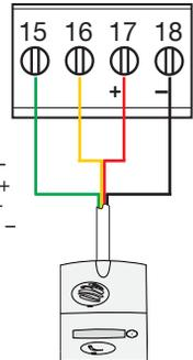
**TIP:** if the cable between the outdoor caller unit and the controller has to be extended, keep or shorten the length of the cable supplied and then connect the wires to a branch box in accordance with the rules below:
