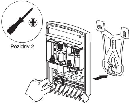
2. Following the installation rules below, mark 3 fixing points and drill a hole in the pillar using a  $\text{Ø } 6 \text{ mm}$  drill bit.
