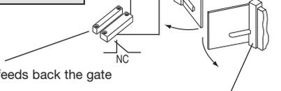
The position contact feeds back the gate status to the screen:
