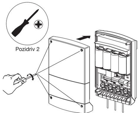
**No reprogramming is required after the batteries have been changed.**
