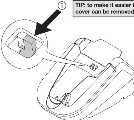
**TIP:** to make it easier to pick the handset up, the removable transparent cover can be removed.
